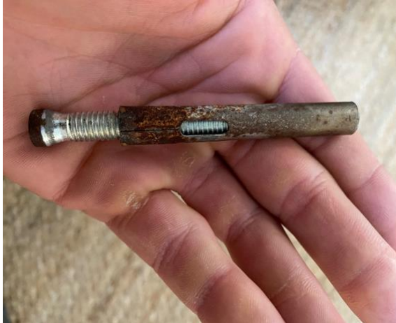
Figure 3: An old \frac{3}{8} inch plated steel bolt that was removed and replaced by a climber in Western Colorado. Note the rust on the bolt sleeve.
